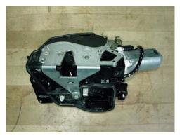
The Drivers lock assembly contains two hall sensors for the signalling of the position of the external lock cylinder in the drivers door. The hall sensors signal:
